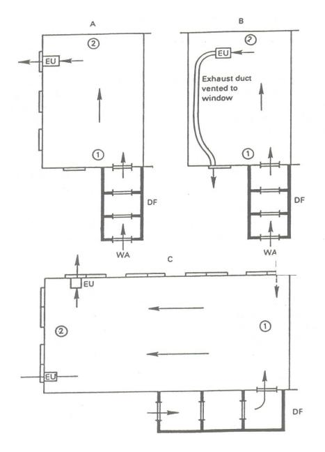
Figure 9-1 Examples of Negative Pressure Systems
