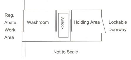
All waste and equipment exiting the work area must pass through the waste decontamination system prior to being removed from the site. External surfaces of asbestos waste bags and wrapped debris, as well as all tools and other equipment must be wet wiped and/or HEPA vacuumed in the work area before being permitted to exit the site.
